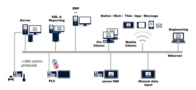
Figure 9: Architecture of an EPS, integrated from production area to ERP level
