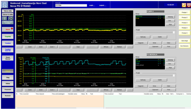
Štrand pumping station: system parameters and measurement of current, pressure and flow.
