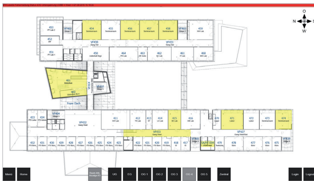
An overview of all rooms on one floor. The individual status is displayed in color schemes.
