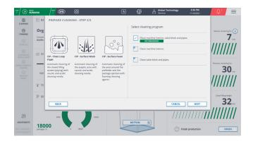
SIG NEO has an automated cleaning feature. The HMI guides users intuitively through the process.
